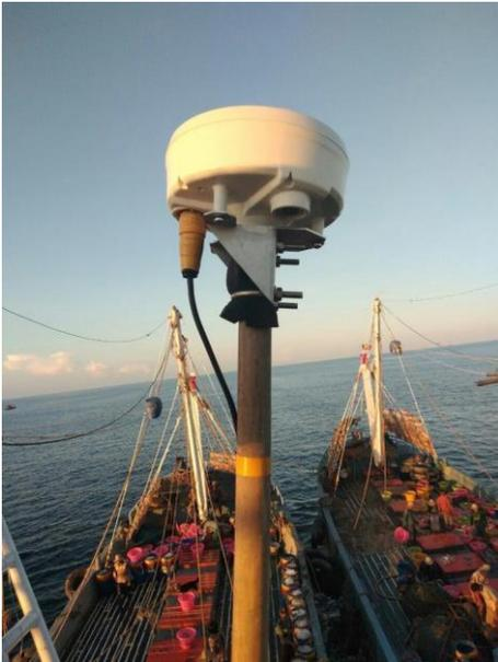
The Triton Advanced Terminal is one of the world's leading Vessel Monitoring Systems (VMS) terminals. It automatically transmits the position, speed, heading and logbook via satellite. It is robust, highly reliable and easy-to-install.
